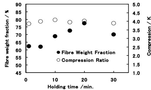
Fig.5. Effect of holding time on the fiber wt. fraction and compression ratio of the bagasse composites.
