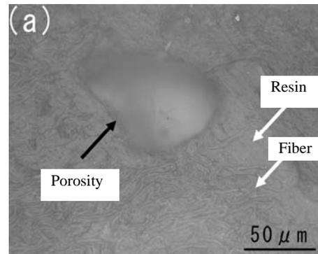
Fig.12a. Optical microphotographs of the cross section of the bagasse composite specimens
