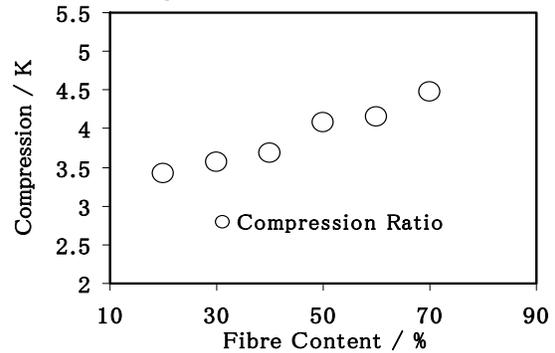
Fig.10. Effect of fiber content on the compression ratio of bagasse fiber composites.
