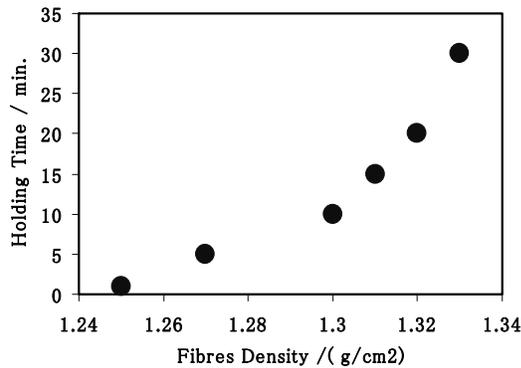
Fig.7. Relationship between holding time and fiber density of the bagasse composites.
