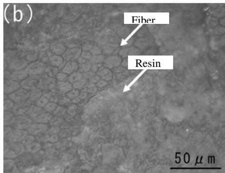
Fig.12b. Optical microphotographs of the cross section of the bamboo composite specimens
