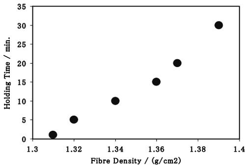
Fig.8. Relationship between holding time and fiber density of the bamboo composites.
