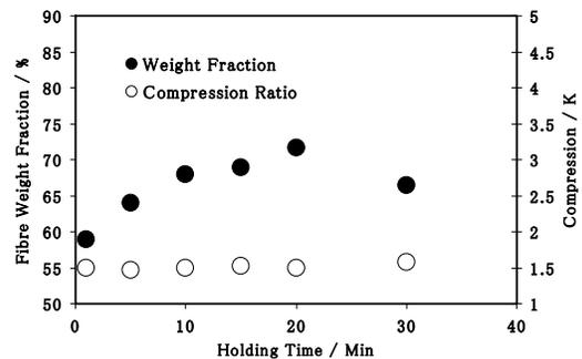
Fig.6. Effect of holding time on the fiber weight fraction and compression ratio of the bamboo composites.
