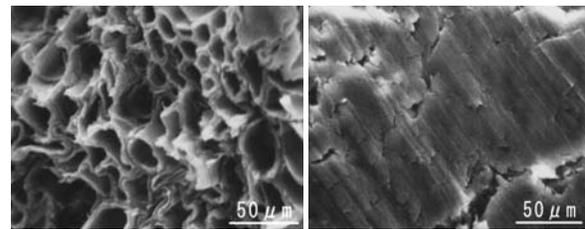
Fig.11. Cross section of a) bagasse fiber and b) bamboo fiber
