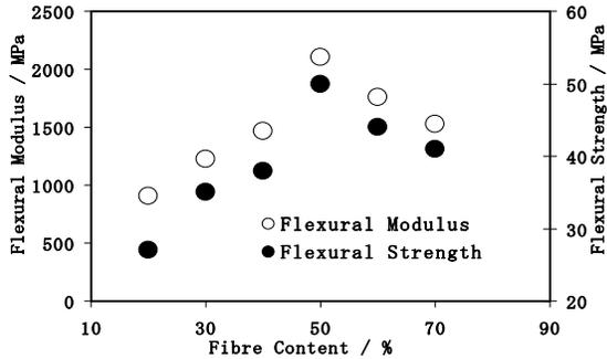
Fig.9. Effect of fiber content on flexural properties of bagasse composites
