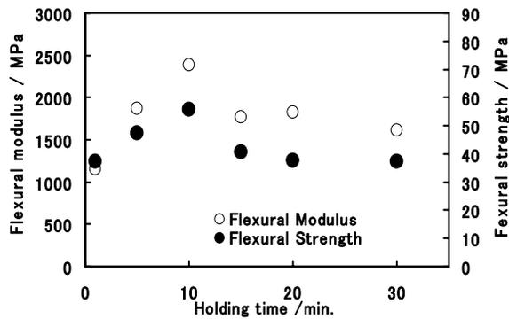
Fig.3. Effect of holding time on the flexural properties of bagasse composites.
