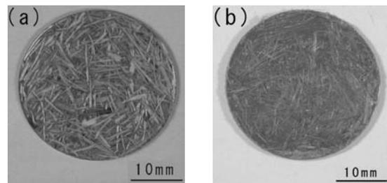
Fig. 1: Press forming with the cylindrical mould, (a) Before moulding, (b) After moulding.
