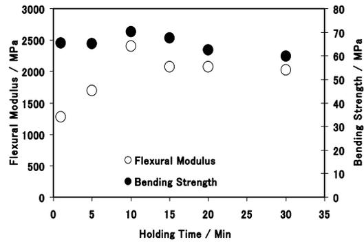
Fig.4. Effect of holding time on the flexural properties of bamboo composites.
